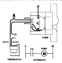
WIRING DIAGRAM FOR THERMOSTATIC CONTROL ONLY
