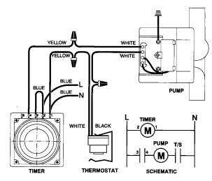
WIRING DIAGRAM FOR TIMER AND THERMOSTAT (Wired in Series)
